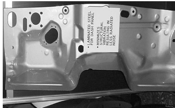
Fig. 8. Damped dash panels using VEM.
